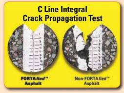
These test samples from the C Line Integral Crack Propagation Test are for a visual comparison of unmodified asphalt, meaning no FORTA-FI fibers, and FORTA fied asphalt mixtures. The test demonstrated that the more energy required and the slower the crack speed, the better the mixture will resist cracking. Fiber-reinforced asphalt controls cracking as seen by additional tests performed at Arizona State University that showed:
