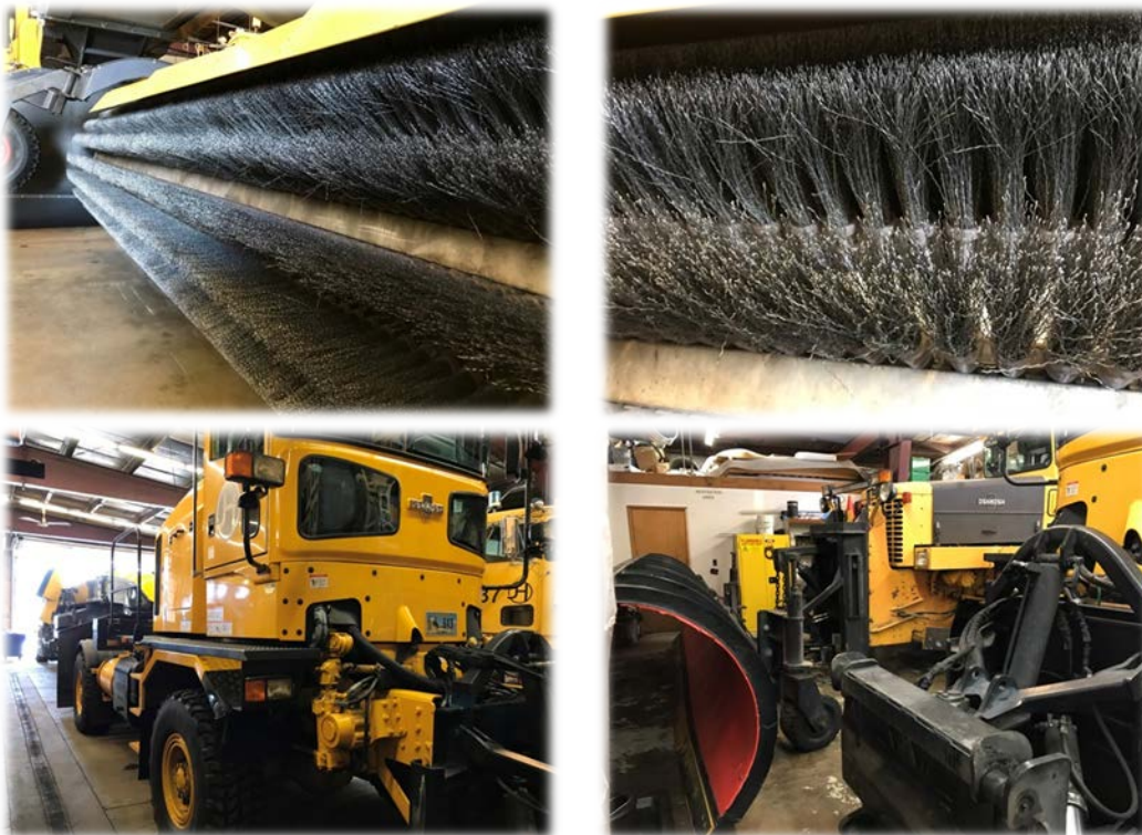
Figure 2. Example steel-bristled brooms and steel-blade snow removal equipment.
