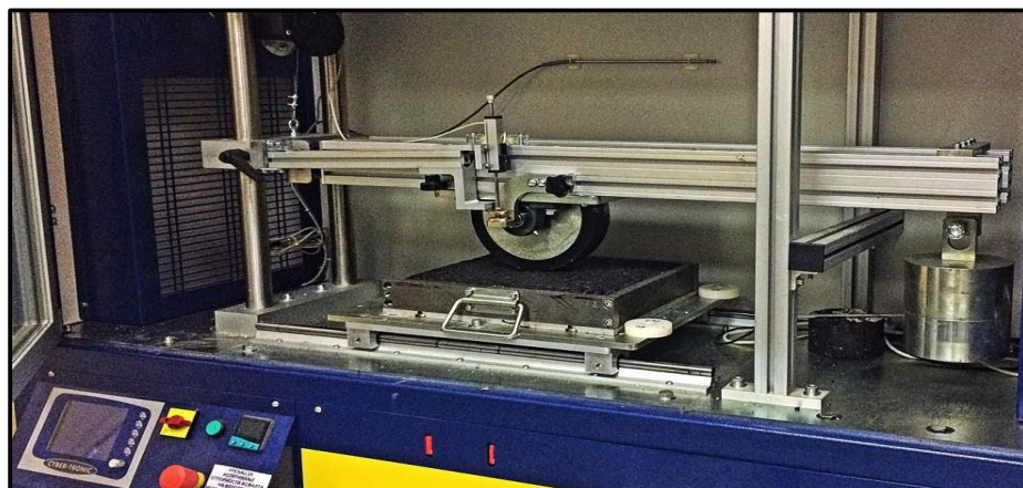
Figure 7. Devices and specimen during the rut testing
