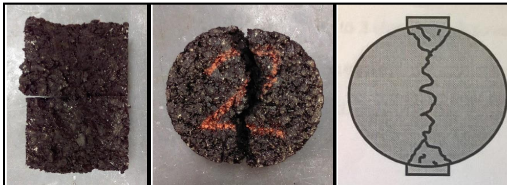
Figure 10. Failure type of specimen of asphalt mixture AB 11s with and without addition of "FORTA-FI®"
