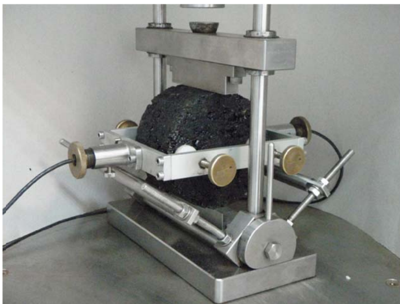
Figure 6.1. Specimen fixed in loading frame during stiffness modulus test in IT-CY scheme
