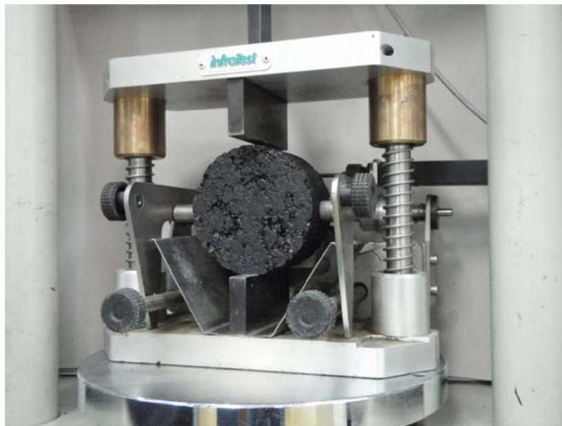
Figure 6.2. Specimen fixed in loading frame for indirect tensile strength test
