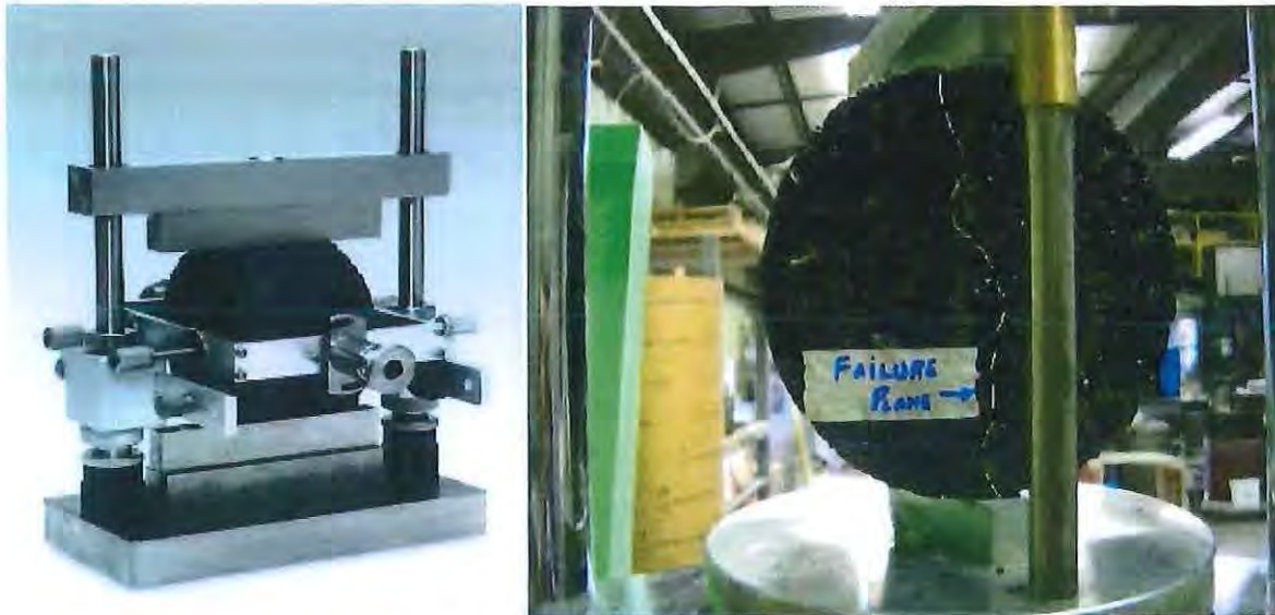
Figure 9: IDT Strength Test Set up and Failure Plane Using Indirect Tensile Jig
