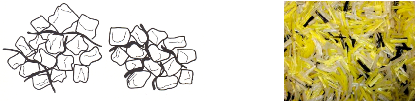
Figure 2 and 3 Dispersion of the fibers in mineral skeleton related to the length of the fiber, mix of FORTA fibers for Hot Mix Asphalt
