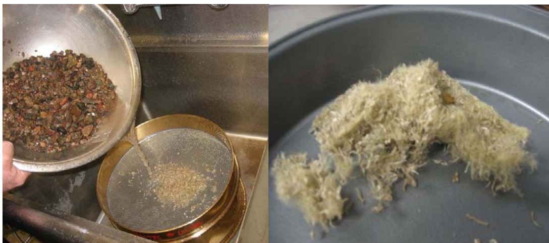
Figure 86 (a) Wet Sieving and Retrieval of the FORTA Fibers (b) Retrieved (Dried) Fibers
