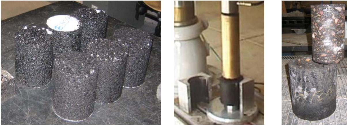
Figure 10 Asphalt Concrete Plug Preparation Procedure
