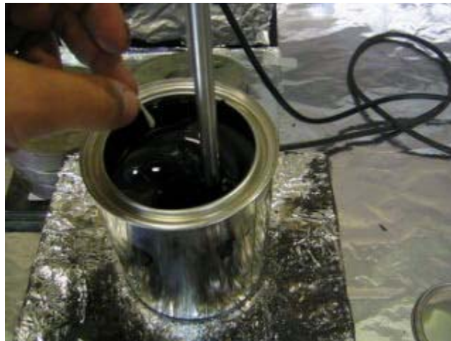
Figure 13 Preparation of Polypropylene Modified Binder
