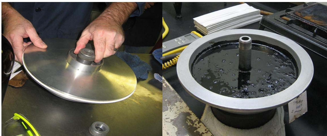
Figure 83 (a) Mix Soaked in Trichloroethylene (b) Mix Bowl (before Keeping in Centrifuge)
