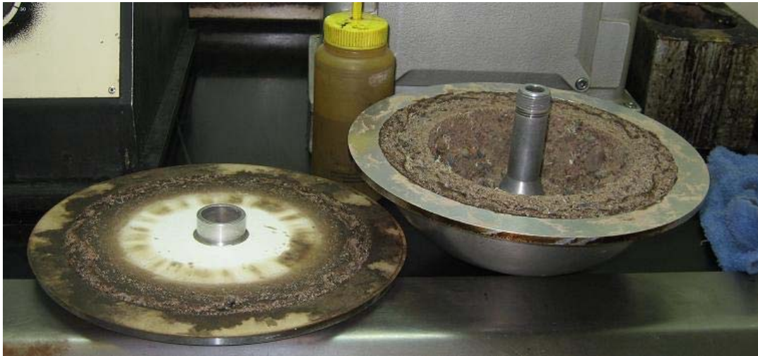
Figure 85 Picture Showing Aggregate and Fibers after Bitumen Extraction
