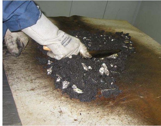
Figure 82 (a) Fiber Soaked in Different Solvents (b) Disintegration of the Asphalt Sample
