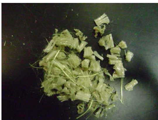
Figure 87 Fibers after Exposing to High Temperature (>160 °C)
